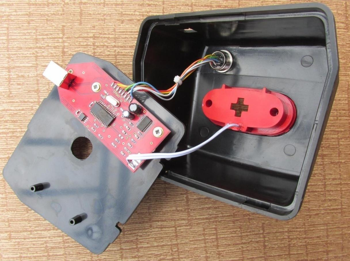
10. Place down cover and fix it in the groove from USB connector side (back side of box).
