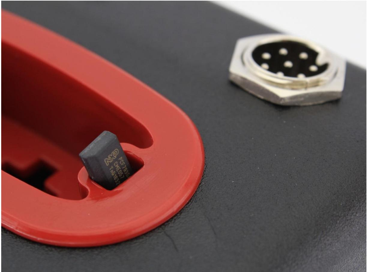
Special place for round shape glass transponder for easy fixing during reading and programming operations.
