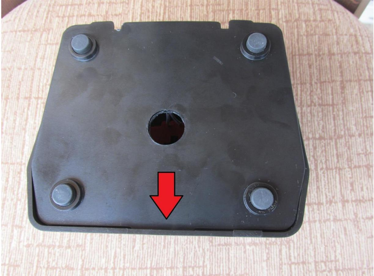
11. Firmly press on both sides of other end of cover (front side of box) till you hear "CLICK" sound from both sides.
