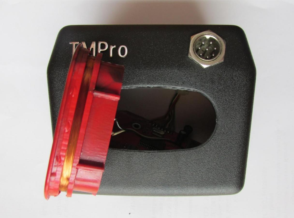
7. Place antenna in hole and firmly press on left and right side till you hear "CLICK" sound.
